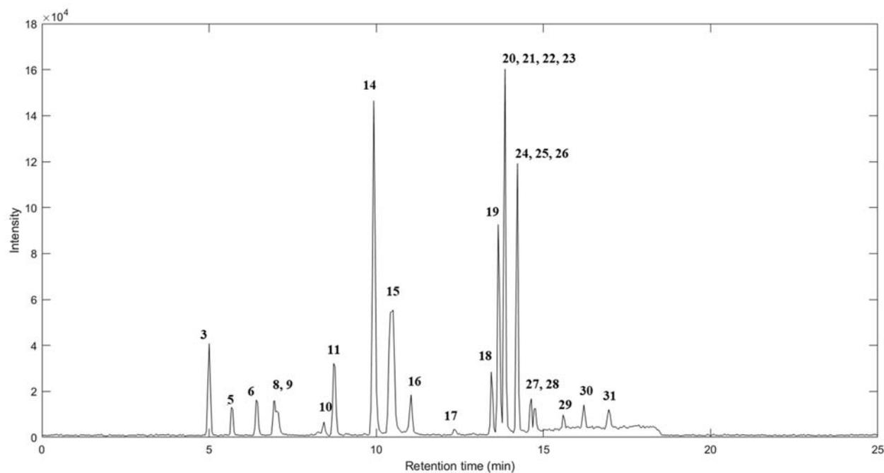
Fig. 1. Total ion chromatogram (TIC) of a sample mixture LC08 using LC-ESI (a) and LC-APCI (b). The label on the peaks and the corresponding structures are listed in Table 1. APCI showed a greater peak area for flonicamid (peak 3) while 8 pesticides including aldicarb sulfoxide, oxamyl, thiamethoxam, butocarboxim, flazasulfuron, bensulfuron-methyl, and fludioxonil (peak 1, 2, 4, 7, 12, 13, and 17), produced no signals in APCI.
