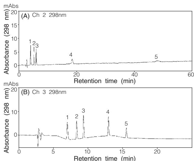
**Figure 3.** HPLC chromatograms of four benzimidazole standards after (A) isocratic elution with acetonitrile/0.01M ammonium dihydrogen phosphate (1/1, v/v), and (B) gradient elution with acetonitrile and 0.01M ammonium dihydrogen phosphate according to the profile described in Table 1.
