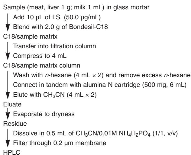
Figure 2. MSPD procedure for four benzimidazole residues.
