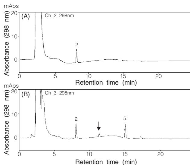
**Figure 4.** HPLC chromatograms of FBT spiked into bovine milk sample at 0.20 ppm using traditional method of extraction. (A) Blank bovine milk, (B) spiked bovine milk, the peak with an arrow was derived from FBT (peak 5). Peak identification is shown in Figure 3.
