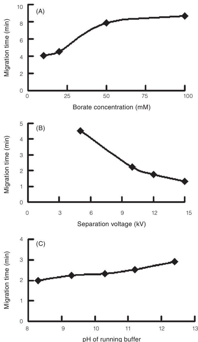
**Figure 3.** Effects of electrophoretic conditions on migration time of OPA-labeled glucosamine. (A) 5 kV, pH 9.3, (B) 20 mM borate buffer, pH 9.3, (C) 20 mM borate buffer, 10 kV. The mixing time was 12 sec; other conditions are as in Figure 1.
