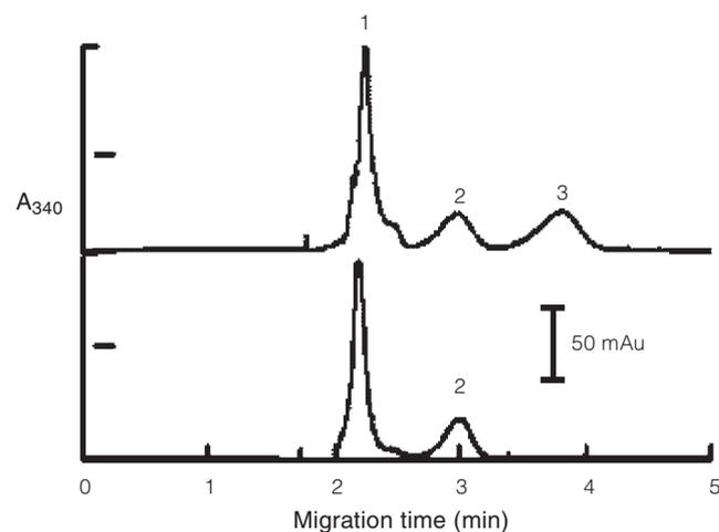
**Figure 4.** Electropherograms of a sample solution (upper trace) and glucosamine standard solution (lower trace). The mixing time was 12 sec; other conditions are as in Figure 1. Peaks 1, 2 and 3 are the signals of OPA-glucosamine, OPA-glycine and an unidentified chemical, respectively. The standard solution contained 20 mM glucosamine and 10 mM glycine.
