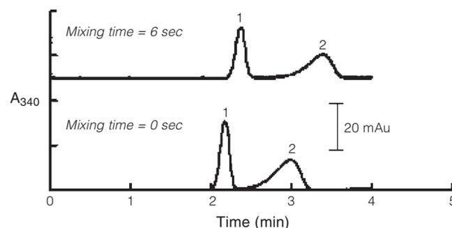
**Figure 1.** Effects of mixing time on electropherogram. Capillary were injected sequentially with OPA reagent (30 mbar  $\times$  5 sec), glucosamine solution (10 mM; 30 mbar  $\times$  3 sec) and OPA reagent (30 mbar  $\times$  5 sec), and then separated (10 kV) with the running buffer of 20 mM borate, pH 9.3.  $A_{340}$  was monitored. The glucosamine (Peak 1) solution contained 5 mM glycine (Peak 2). Other conditions are detailed in the experimental section.
