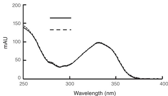
**Figure 5.** Comparison of the absorption spectra. Spectra of peak 1 (OPA-glucosamine) in Figure 4 were obtained with the built-in PDA detector of the CE machine. Solid line: glucosamine standard; dashed line: sample solution of a nutraceutical.
