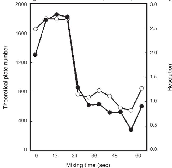
**Figure 2.** Effects of mixing time on the theoretical plate numbers and resolutions of electropherograms. The experimental conditions are shown in Figure 1. Open circles: theoretical plate numbers; solid circles: resolutions.
