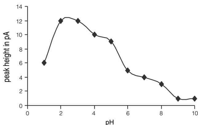
**Figure 2.** Effect of pH on the GC elution of FAA-INH derivative. GC conditions: The column HP-5 (30 m  $\times$  0.32 mm) with film thickness 0.25  $\mu$ m at an initial column temperature 100°C with heating rate 30°C up to 280°C. The run time was 7 min. Nitrogen flow rate was 1 mL/min and split ratio 20:1. Injection port and detector temperatures were 200°C and 300°C. Nitrogen make up flow rate was 45 mL/min. FID air and hydrogen flow rates were 450 mL and 40 mL respectively.
