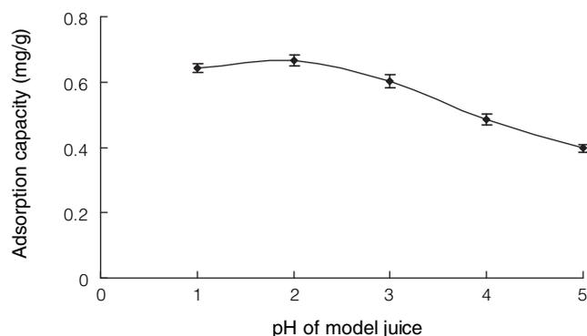
**Figure 2.** Influence of model juice pH on the adsorption capacity of Amberlite IR120 resin. Fifteen milliliter of model juice was mixed with 5 g pretreated Amberlite IR120 resin. The mixture was shaken at 95 rpm at room temperature. Data are expressed as means  $\pm$  standard deviation ( $n = 4$ )  $P \leq 0.05$ .
