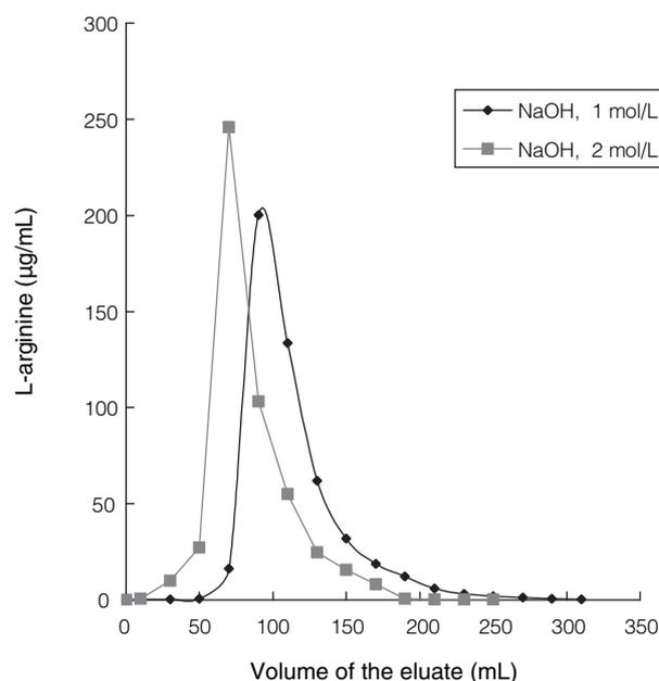
**Figure 4.** The elution curves of model juice in Amberlite IR120 column with NaOH solution. The weight of Amberlite IR120 resin was 16 g. Model juice (10.0 mL, pH 2.0) was loaded to the column at the rate of 0.5 mL/min, and rinsed with distilled water, and then eluted with NaOH solution at the rate of 2.0 mL/min.
