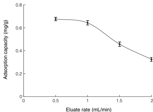
**Figure 3.** Influence of the model juice flow rate on the adsorption capacity of Amberlite IR120 resin. Sixteen gram pretreated Amberlite IR120 resin was packed in the chromatographic column (D 1.0  $\times$  30 cm). The pH of model juice was 2.0. Data are expressed as means  $\pm$  standard deviation ( $n = 4$ )  $P \leq 0.05$ .
