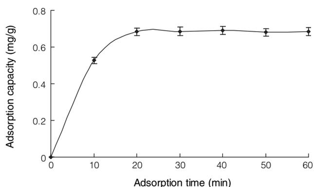
**Figure 1.** Static adsorption curve of arginine by Amberlite IR120 resin. Fifteen milliliter of model juice (pH 2.0) was mixed with 5 g pretreated Amberlite IR120 resin. The mixture was shaken at 95 rpm at room temperature. Data are expressed as means  $\pm$  standard deviation ( $n = 4$ )  $P \leq 0.05$ .
