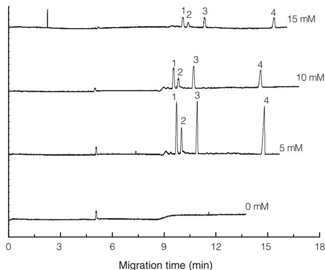
**Figure 4.** Effect of the SDS concentration on the peak area. 1: GV; 2: MG; 3: LMG; 4: LGV. Analytical conditions: 50 mM  $H_3PO_4$  buffer at pH 2.0. Other conditions were similar to Figure 2.
