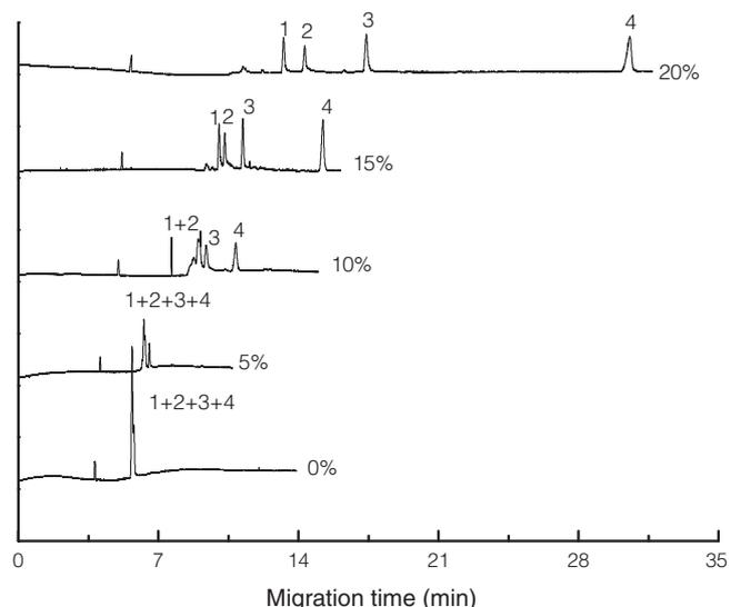
**Figure 3.** Effect of the 2-propanol concentration on the migration time. 1: GV; 2: MG; 3: LMG; 4: LGV. Analytical conditions: 140 mM SDS, 15% acetonitrile. Other conditions were similar to Figure 2.
