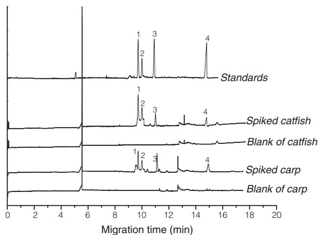
**Figure 6.** Electropherograms of the extract of blank and spiked catfish and carp. 1: GV; 2: MG; 3: LMG; 4: LGV. Analytical conditions were similar to Figure 5A. The analytes of 1 µg/mL (final concentration) were added to the catfish and carp.
