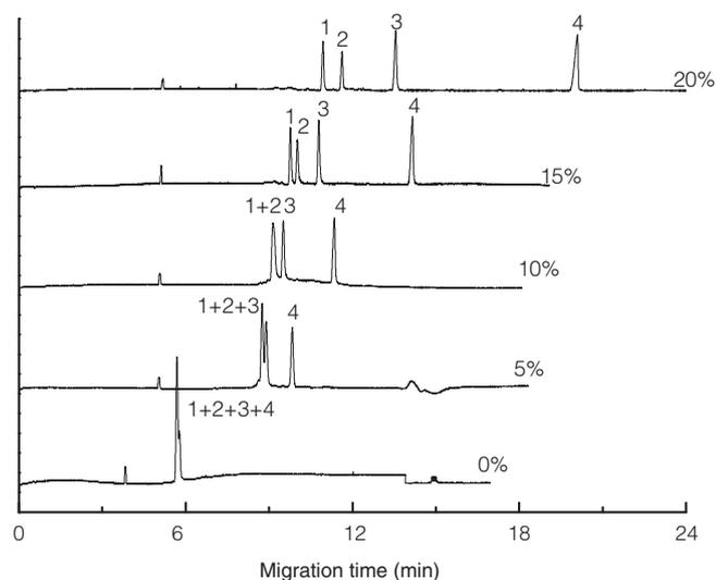
**Figure 2.** Effect of the acetonitrile concentration on the migration time. 1: GV; 2: MG; 3: LMG; 4: LGV. Analytical conditions: 140 mM SDS.
