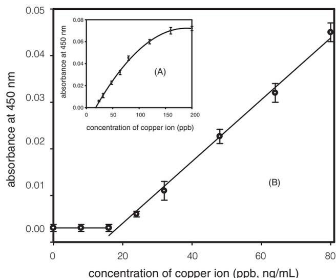
**Figure 4.** Calibration curve for Cu ion (II) determination by the enzymatic method. 10 microliter of apo-SOD (original SOD activity was 20 U) were added into the microplate wells, together with 50  $\mu\text{L}$  of potassium phosphate buffer (30 mM, pH 5.9) and 20  $\mu\text{L}$  of Cu (II) at concentrations ranges of 20 - 80 (A) and 20 - 200 ppb (ng/mL) (B) for 20 min, followed by the determination of SOD activity.
