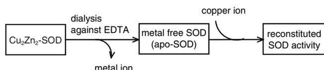
**Figure 1.** The principal mechanism of current assay for the determination of copper ion in aqueous solution.
