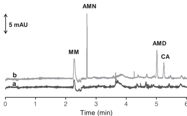
**Figure 4.** Electropherogram of (a) milk chocolate wafer, and (b) milk chocolate wafer spiked with melamine (2 mg/L), ammeline (2 mg/L), ammelide (1 mg/L) and cyanuric acid (2 mg/L). Other conditions were similar to Figure 2.
